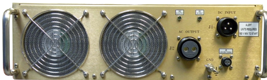
Typical Rear View – 19" Rack Mount Chassis Configuration
