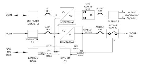
Inverter Mode Functional Block (DC-AC): The 28VDC Battery Input is applied to DC IN J5(+) / J6 (-) Connectors, EMI Filter, DC IN CB1 Breaker, A1 3KW Inverter Module (converts 28VDC to 220VAC 60Hz 13.6A / 230VAC 50Hz 13.04A Max.) and then to Transfer Switch Relay K1. This is followed by AC OUT CB4 Breaker and AC OUT Connectors J1 / J2.
