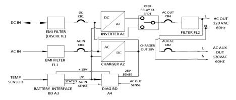
Inverter Mode Functional Block (DC-AC): The 24VDC Battery Input is applied to DC IN J5(+) /J6 (-) Connectors, EMI Filter, DC IN CB1 Breaker, A1 3KW Inverter Module (Converts 28VDC to 120VAC 60Hz 25A max,) and then to Transfer Switch Relay K1. This is followed by AC OUT CB4 Breaker and AC OUT Connectors J1 / J2. The AC OUT is also tapped off and provided to AUX AC CB2 and to AC AUX OUT (p/o J3 Connector.)
